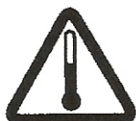
Hot surface warning
